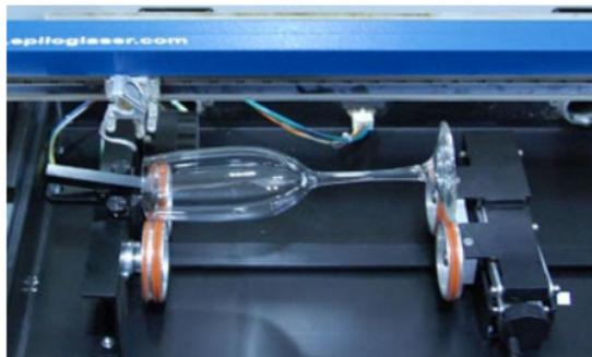
Cylindrical objects can be fixed and machined via an additional rotary device which is secured into the laser bed.
